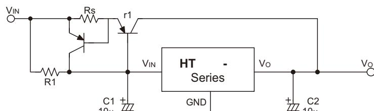
**Circuit for Increasing Output Voltage**
