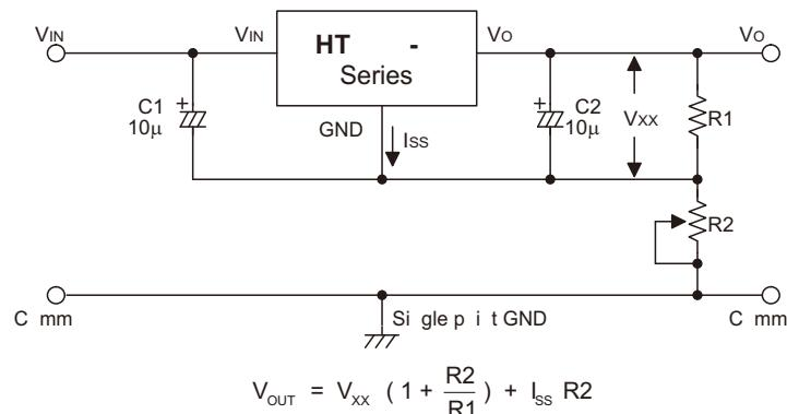
**Circuit for Increasing Output Voltage**
